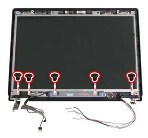
5. Disconnect the two connectors on either side of the inverter board. Remove the inverter board.
