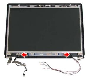
6. Gently lift out the display. Remove the eight M2x3 screws securing the hinges to the display.
