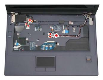
2. Remove the four M2.5x4 screws securing the LCD module to the logic upper.
