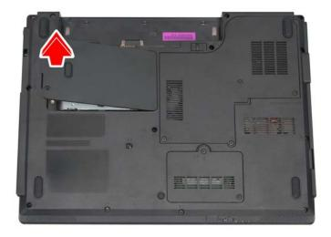
4. Remove the two M2.5x4 screws securing the HDD module in place.
