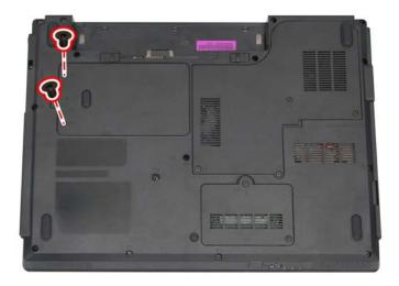
3. Pull up the HDD compartment cover in the direction of the arrow.
