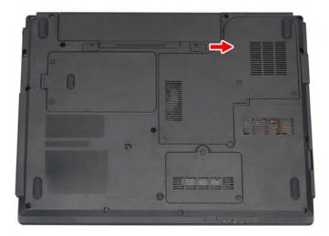
3. Slide the left battery release latch in the direction of the arrow. The battery pack will pop-up automatically. Gently pry the battery pack from its housing.
