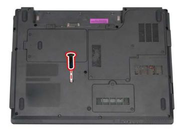
3. Insert a flat screwdriver into the slot as shown and gently push out the ODD.
