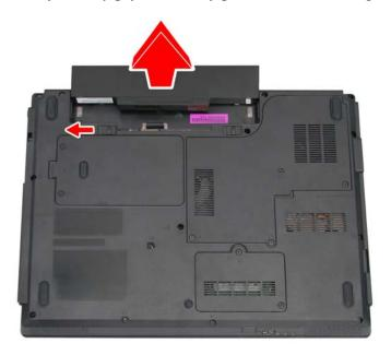
**NOTE**: Always start laptop disassembly by removing the battery pack first.
