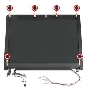
2. Remove the six M2.5x6 screws securing the LCD bezel to the LCD module.
