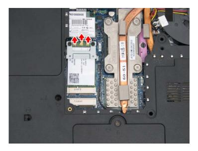
4. Remove the two M2x3 screws attaching the stand-off bracket to the motherboard.
