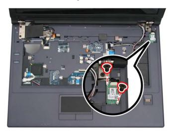
2. Disconnect the Bluetooth cable, and remove the Bluetooth module.
