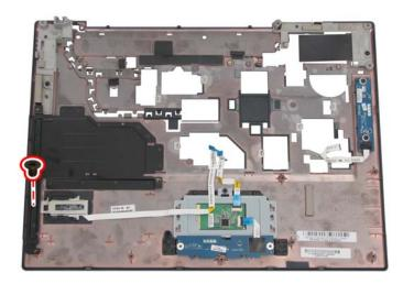
2. Remove the fingerprinter module.
