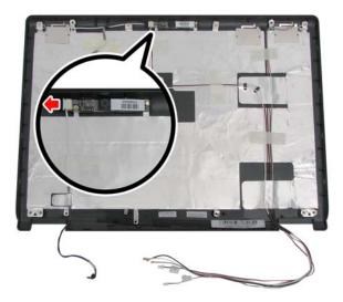
2. Remove the M2x3 screw securing the camera module to the LCD cover. Remove the camera module.
