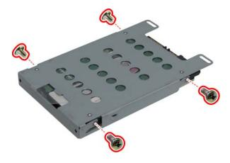
7. Remove the HDD module from the HDD case.
