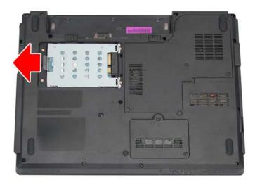
6. Remove the four silver M3x3 screws to take off the HDD case.
