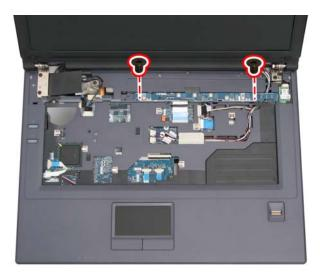
2. Remove the switch board.
