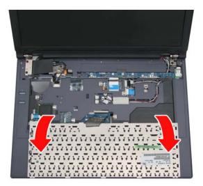
4. Use a thin tool such as a screwdriver to lever up the connector bracket and disconnect the keyboard cable from the motherboard.
