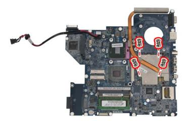
2. Remove the VGA heat sink.
